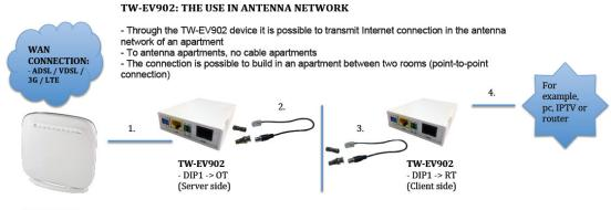
Modem (for example TW-EAV510) makes the WAN connection
